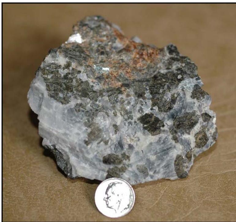
Figure 2. Augite skarn (9 cm): augite, garnet, bluish-gray calcite, trace sphalerite (above dime). University of Delaware specimen, Sharon Fitzgerald photo.
